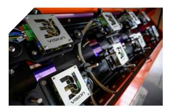
**High resolution, multispectral, 4 wavelength cameras SWIR (1024 pixel):** These cameras achieve previously unattainable results in the recognizing of polymers, selecting of shell and foreign bodies in dried fruits, and also in detecting chemical differences not visible to the human eye.
